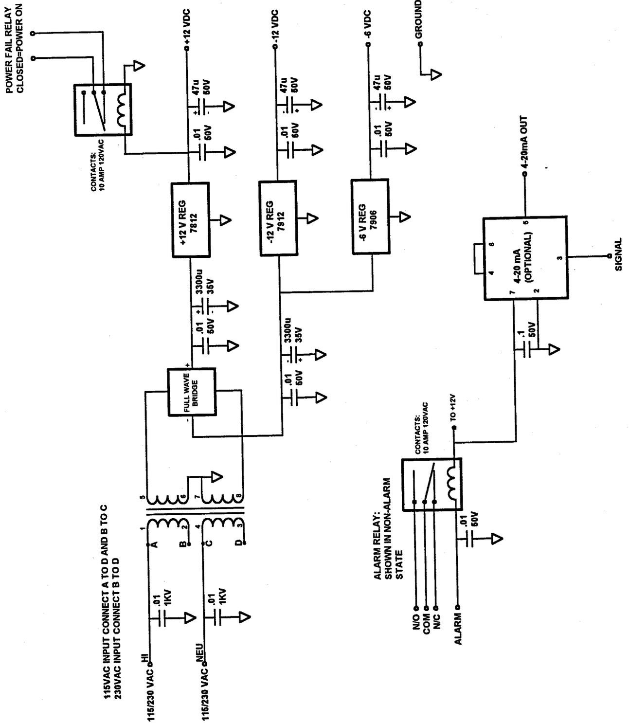
Figure 10 BA-200 Power Power Supply Card
