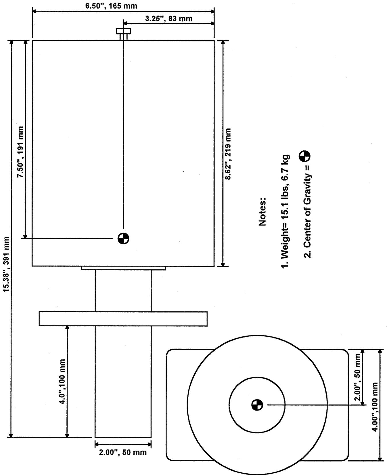
Figure 1 BA-200 Center of Gravity
