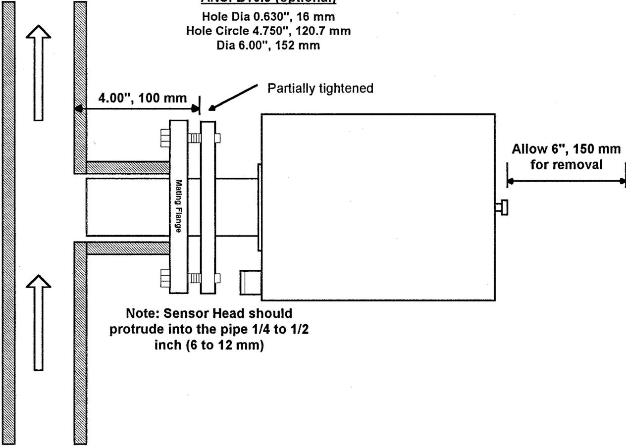
**Note: Sensor Head should protrude into the pipe 1/4 to 1/2 inch (6 to 12 mm)**
